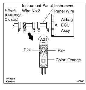
Measure the voltage according to the value(s) in the table below when the power switch is on (IG).
