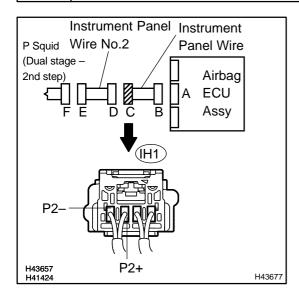
(a) Disconnect the instrument panel wire connector from the instrument panel wire No.2.
