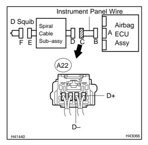
(a) Disconnect the instrument panel wire connector from the spiral cable sub–assy.
