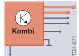
The instrument cluster has no gateway function as on the previous model variants.
