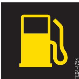
Indication of the fuel reserve is an integral part of the on-board computer and is not represented as an analogue gauge in the instrument cluster.
