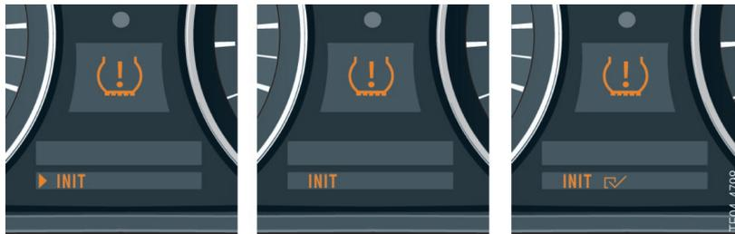
2 - Initialization of the tyre failure indicator RPA
