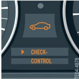
A graphic symbol in the upper display window is assigned to each main menu item. Menu items that are deactivated during vehicle operation are not shown.
