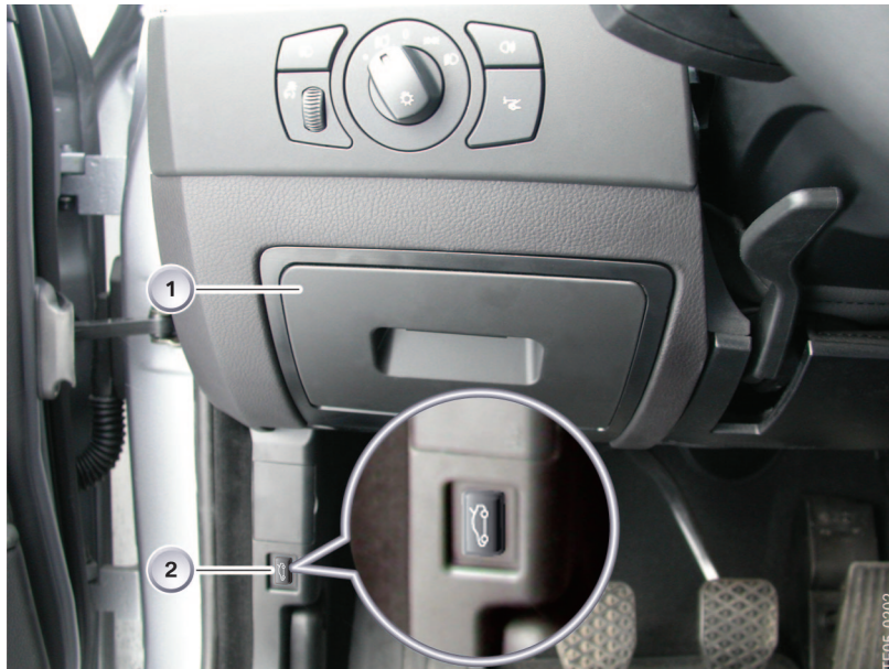
6 - Storage compartment is larger and lockable. Boot lid can be opened by means of a button in the vehicle interior.
