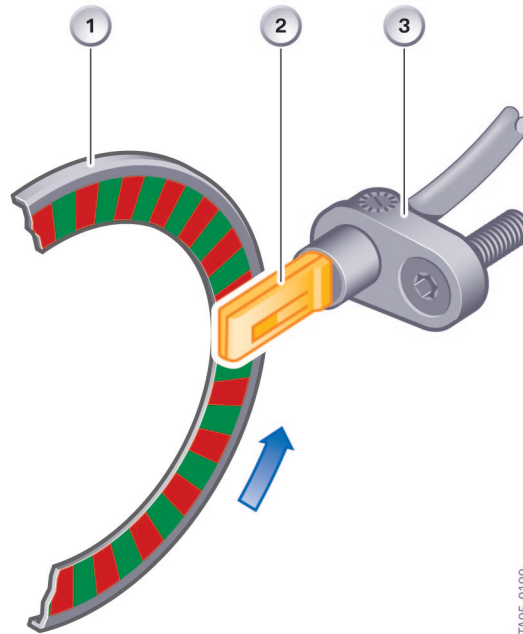
8 - Wheel speed sensor with sensor ring
