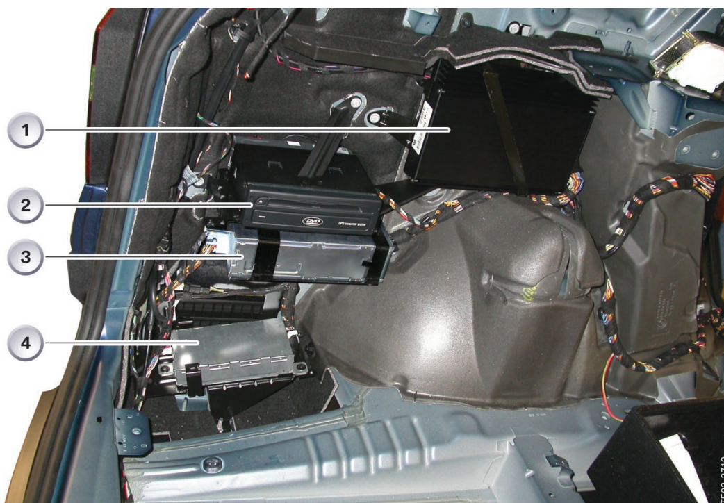
Fig. 70: Installation location video module (position 3)
