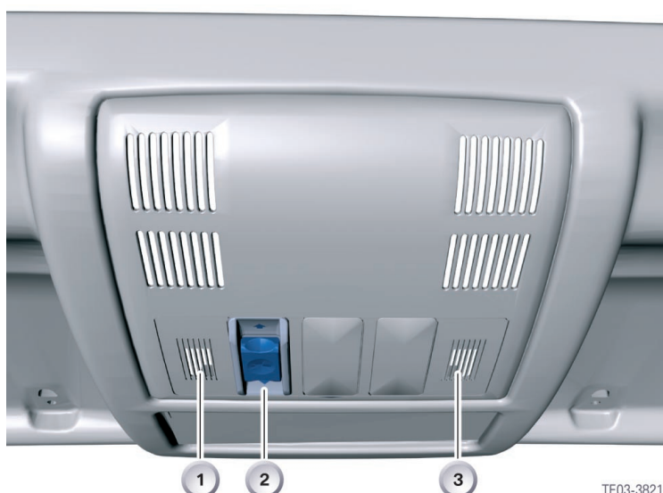
Fig. 31: Hands-free microphone in the roof console
