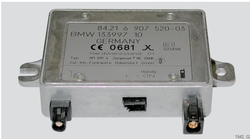
Fig. 41: Aerial line compensator for the ULF
