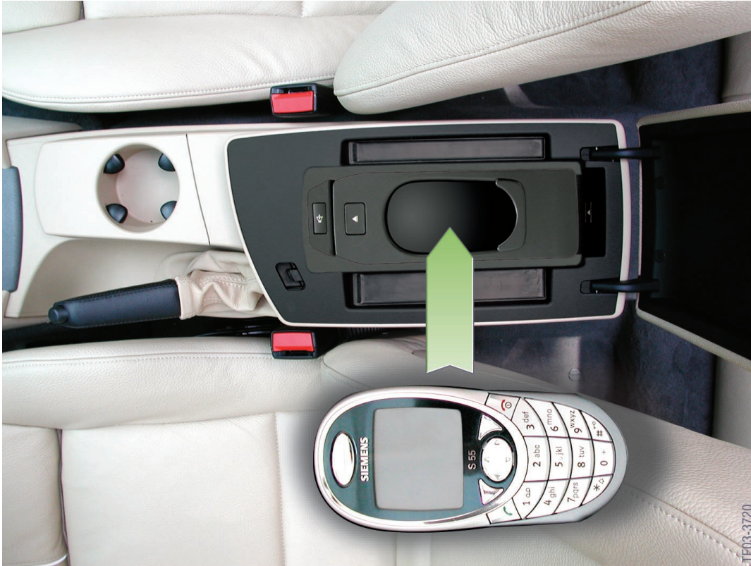
Fig. 40: Snap-in adapter with Siemens S55 mobile phone
