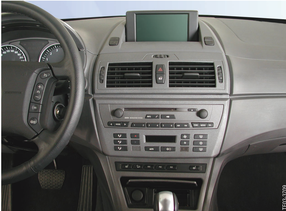
Fig. 8: Installation location of the BMW CID radio (option 609)
