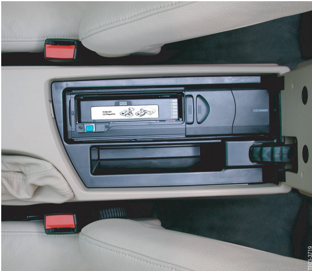
Fig. 10: Installation location of the CD changer between the front seats
