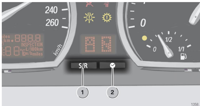
Fig. 9: Setting buttons in instrument cluster
