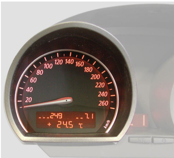
Fig. 16: E85 Example: test function outside temperature (test function 71)
