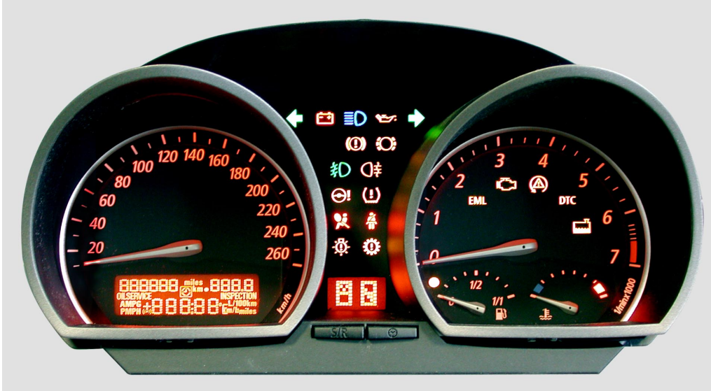
Fig. 17: E85 Test function 2, visual system test
