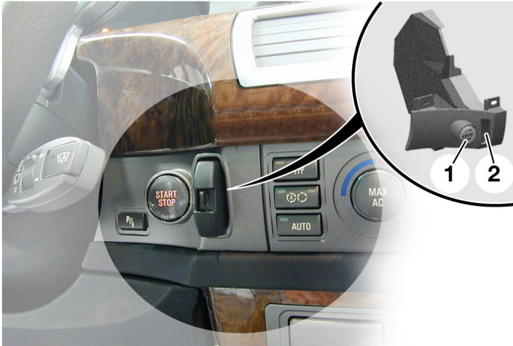
Fig. 3: Ignition switch and starter/stop button
