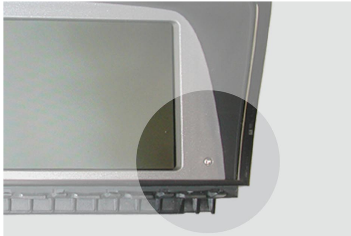
Fig. 23: Photoelectric cell in LCD display unit
