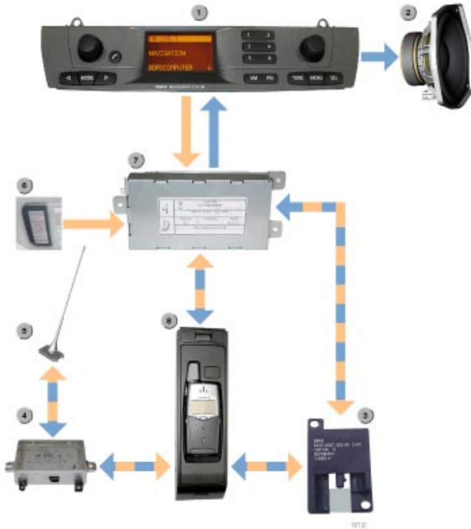
Fig. 4: System overview of universal charging and hands-free unit ULF
