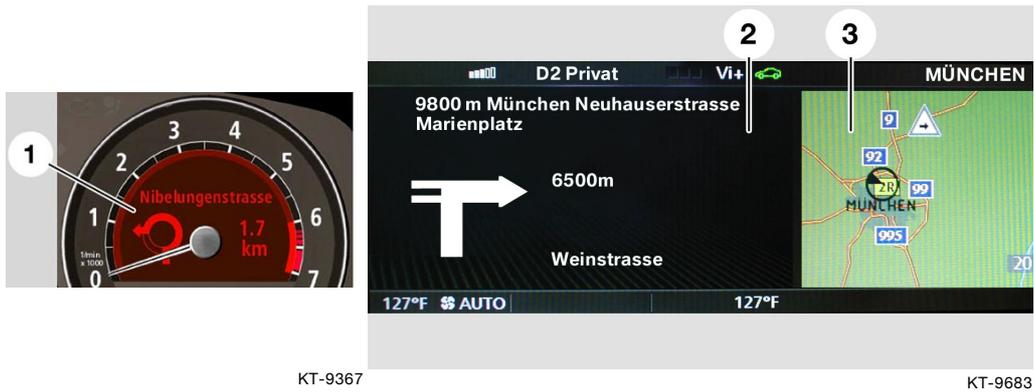
Fig. 1: Example of the navigation display in the instrument cluster and in the control display
