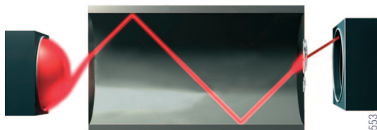
6 - Soiled end faces of fibre optics conductor
