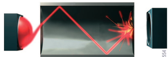
7 - Scratched end faces of fibre optics conductor
