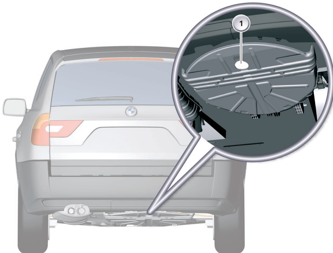
Fig. 10: Service opening (1) in the compact wheel bracket
