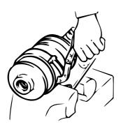
Water level sensor With holding water level sensor in vice, turn and remove the fuel filter cartridge with both hands.
