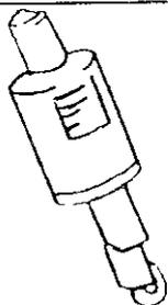
Figure 1. Late style timing connector.
