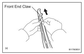
(d) Slide the wiper rubber through the front end claw.
