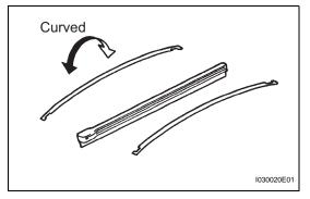
(b) Remove the wiper blade as shown in the illustration.
