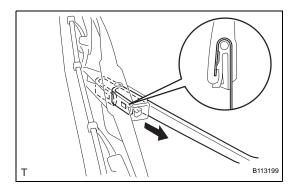
(b) Install the wiper rubber to the claw of the wiper blade in the direction indicated by the arrow in the illustration.
