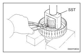
(c) Place SST on the clutch balancer and compress the piston return spring with a press.
