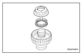
(b) Install the piston return spring and clutch balancer to the underdrive clutch drum.
