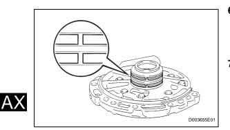
6. INSTALL CLUTCH DRUM OIL SEAL RING NOTICE: Do not expand the ring ends excessively
