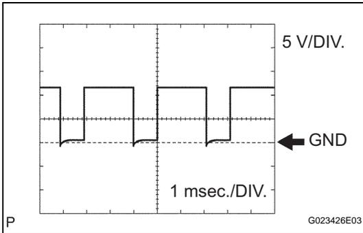
(c) Using an oscilloscope, check the waveform 2.
