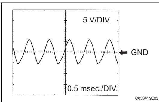
(f) Using an oscilloscope, check the waveform 5.
