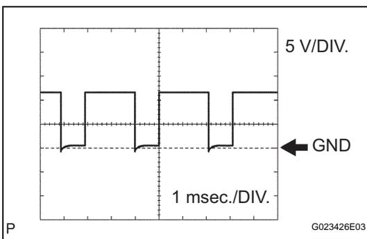
(e) Using an oscilloscope, check the waveform 4.
