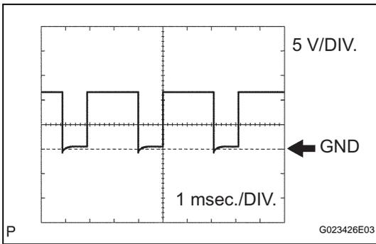
(b) Using an oscilloscope, check the waveform 1.
