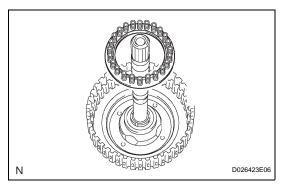
(d) Remove the overdrive clutch return spring from the direct clutch drum.
