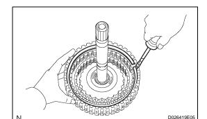
(b) Remove the flange, 3 discs, 3 plates and cushion plate from the intermediate shaft.
