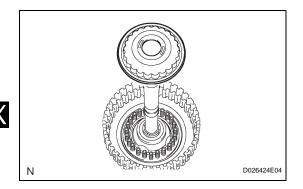
(c) Remove the clutch balancer from the direct clutch drum.
