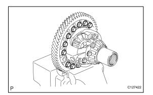
(f) Remove the 16 bolts and the transaxle housing.
