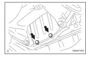
(d) Install the flywheel housing under cover with the 2
