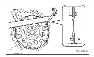
(c) Using a vernier caliper and straightedge, measure dimension B shown in the illustration and check that B is greater than A.
