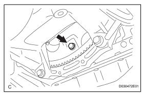
(c) Install the 6 torque converter clutch mounting bolts.
