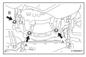
(b) Install the 3 lower side mounting bolts.
