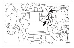
(c) Install the terminal nut and cover the nut with the cap.
