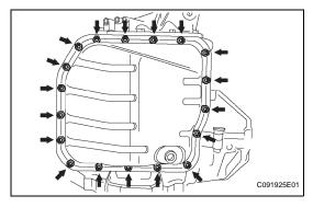
(b) Install a new gasket and the oil pan with the 18 holts
