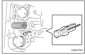
(b) Remove the check ball body and spring.
