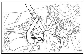
(d) Remove the bolt and disconnect the clamp of the control cable.
