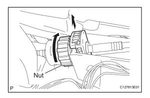
f) Turn the nut and disconnect the control cable from the shift lever retainer.
