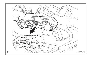
(e) Disconnect the control cable from the shift lever.
