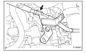
(h) Connect the control cable to the cable support.
