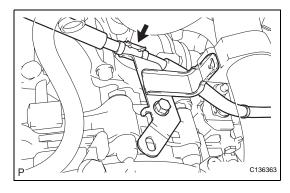
(c) Disconnect the control cable from the control cable support.
