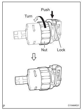
(b) Turn the nut of the control cable and push in the lock.
