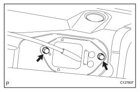
(g) Remove the 2 bolts and control cable.
