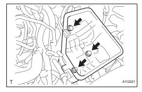
(b) Install the air cleaner case with the 3 bolts. Torque: 5.0 N\*m (51 kgf\*cm, 44 in.\*lbf)
