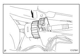
(c) Install the control cable onto the shift lever retainer.
