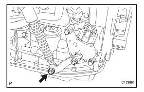
(f) Connect the control cable onto the control shaft lever with the nut.
