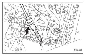
(e) Fix the control cable onto the control cable bracket with the clip.
