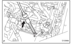
(b) Remove the clip and disconnect the control cable from the control cable bracket.
