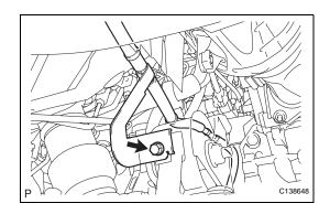
(g) Connect the clamp of the control cable with the bolt.
