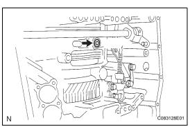
(b) Install the piston to the transaxle case and coat the piston with ATF.
