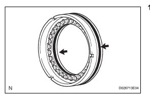
(c) Using a snap ring expander, install the snap ring. **NOTICE:**
