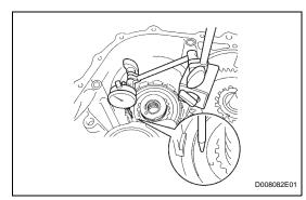
(c) Using a screwdriver, install the snap ring.NOTICE:The snap ring should be fully engaged in the
