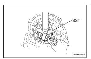
(c) Coat the 1st and reverse brake piston with ATF, and install it to the transaxle case.
