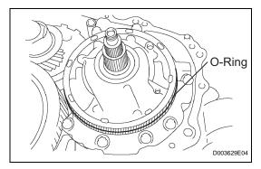
(b) Coat the O-ring of oil pump with ATF.
