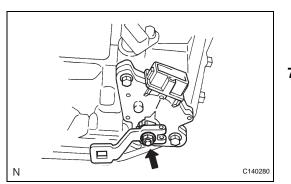
(j) Install the control shaft lever with the washer and nut.
