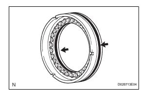
(b) Remove the 2 O-rings from the 1st and reverse brake piston.
