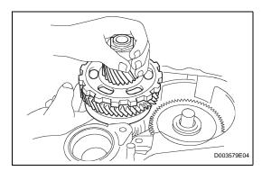
(d) Remove the underdrive planetary gear from the transaxle case.
