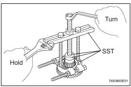
(c) Using SST, remove the tapered roller bearing.
