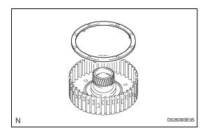
(c) Remove the planetary carrier thrust washer from the rear planetary sun gear.
