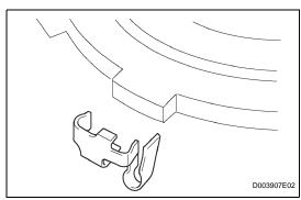
(c) Remove the outer race retainer from the 1-way clutch.
