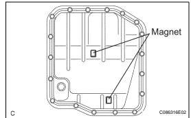
(b) Remove the 2 magnets from the oil pan.
