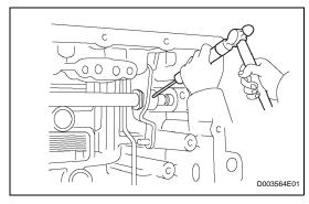
(b) Using a pin punch (φ35 mm) and hammer, drive out the pin.
