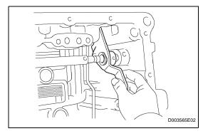
(c) Remove the manual valve lever shaft and manual valve lever.
