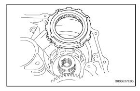
(b) Remove the underdrive 1-way clutch from the transaxle case.
