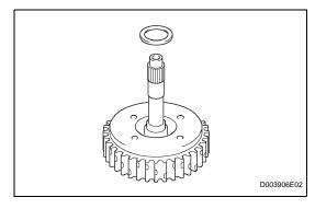
(b) Remove the thrust needle roller bearing from the forward clutch.
