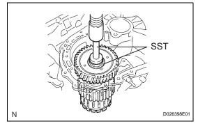
(c) Using SST and a press, press out the front planetary gear from the counter drive gear.
