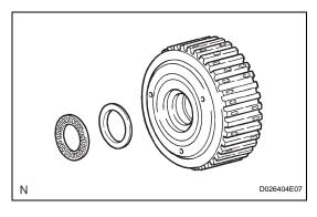
(b) Remove the thrust needle roller bearing and thrust bearing race from the rear planetary sun gear.
