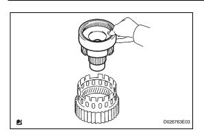
(d) Remove the front planetary gear from the brake hub.
