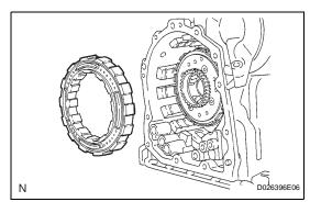
(b) Remove the 2nd brake piston from the transaxle case.
