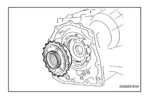
(b) Remove the rear planetary gear from the transaxle case.
