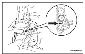
(b) Apply compressed air (392 kPa, 4.0 kgf/cm<sup>2</sup>, 57 psi) to the oil hole and remove the C-3 accumulator piston.
