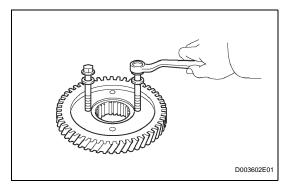
(b) As shown in the illustration, tighten the 2 bolts evenly and make a clearance of approximately. 20.0 mm (0.787 in.) between the counter drive gear and the inner race.
