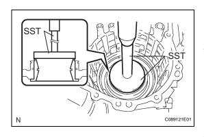
(b) Using SST and a press, remove the bearing outer race.
