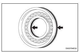
(b) Remove the 2 O-rings from the underdrive brake piston.
