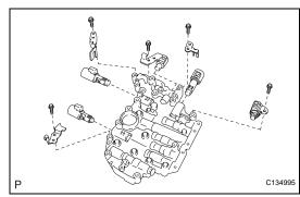
(c) Remove the 5 bolts, 4 plates and 5 shift solenoid valves.
