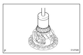
(b) Using a chisel and a hammer, stake the differential case.
