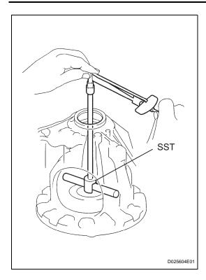
(d) Using SST, return the differential assembly right and left 2 or 3 times to allow the bearing settle.
