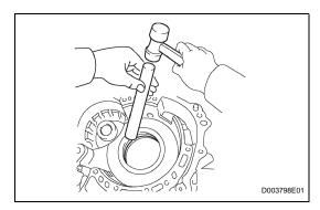
(d) Using a brass bar and hammer, tap out the 2 bearing outer races.
