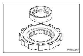
(b) Remove the inner race from the 1-way clutch.
