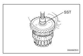
(c) Using SST and a press, remove the front planetary gear from the counter drive gear.
