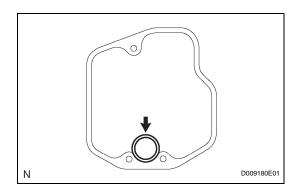
(b) Remove the O-ring from the oil strainer.
