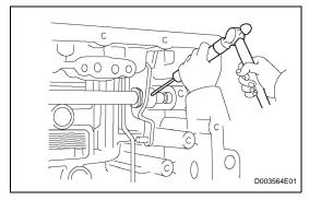
(b) Using a pin punch and hammer, tap out the pin.
