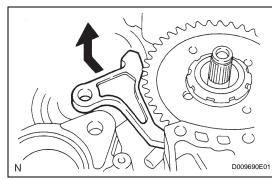
(e) Remove the spring, pawl pin and parking lock pawl.
