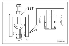
(e) Using SST, remove the needle-roller bearing from the transaxle rear cover.
