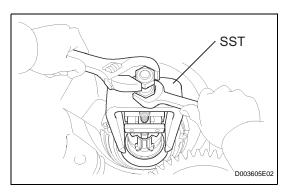
(c) Using SST, remove the needle-roller bearing from the transaxle.
