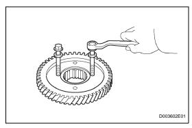
(b) As shown in the illustration, tighten the 2 bolts evenly and make a clearance of approximately 20.0 mm (0.797 in.) between the counter drive gear and the inner race.
