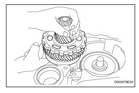
(d) Remove the underdrive planetary gear from the transaxle.
