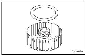
(c) Remove the No. 1 thrust washer from the rear planetary sun gear.
