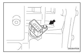
(c) Remove the bolt and transaxle wire.
