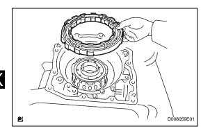
(b) Remove the 2nd brake piston from the transaxle.
