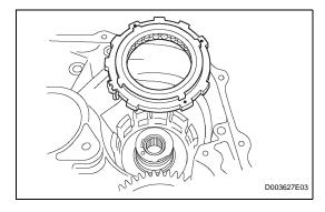
(b) Remove the 1-way clutch from the transaxle.
