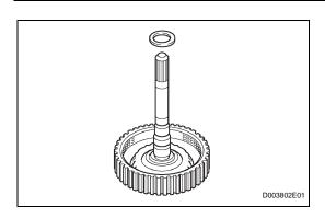
(b) Remove the bearing race from the direct clutch.
