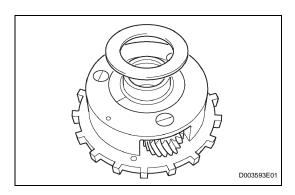
(d) Remove the bearing race from the rear planetary gear.
