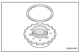
(c) Remove the No. 1 planetary carrier thrust washer from the rear planetary gear.
