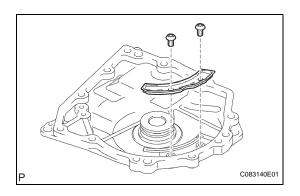
(d) Using a T30 "torx" socket wrench, remove the 2 screws and transaxle rear cover plate.
