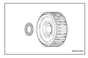
(b) Remove the thrust bearing from the rear planetary sun gear.
