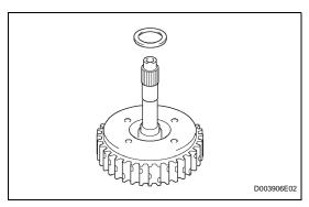
(b) Remove the thrust bearing from the forward clutch.
