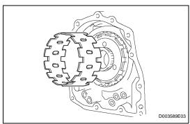
53. REMOVE 1-WAY CLUTCH OUTER SLEEVE
