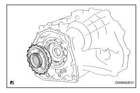
(b) Remove the rear planetary gear from the transaxle.
