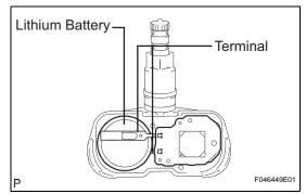
(b) The battery and base board covered with silicone resin are exposed. While taking out the battery, cut the 2 terminals that connect the battery and the base board.
