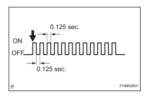
(e) Confirm that the tire pressure warning light in the combination meter blinks at 0.125 second intervals.
