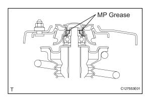
(c) Pack the suspension support with MP grease.
