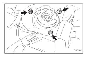
(b) Remove the 3 nuts and shock absorber with coil spring.
