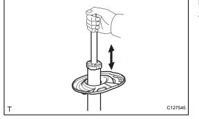
(a) Compress and extend the shock absorber rod 4 times or more. Check that there is no abnormal resistance or unusual sound during the operation. If there is any abnormality, replace the shock absorber assembly with a new one.
