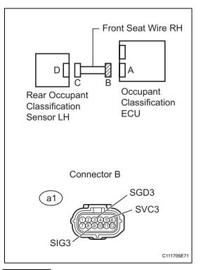
Measure the resistance of the wire harness side connector.
