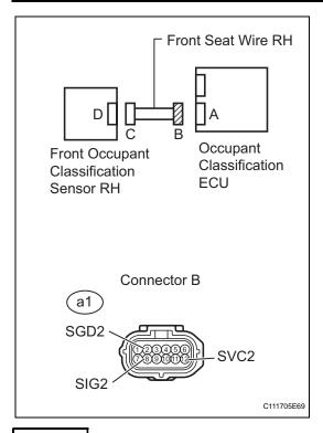
(a) Measure the resistance of the wire harness side connector.
