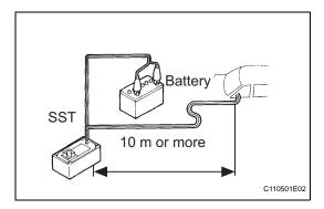
(2) After connecting SST to each other, connect them to the curtain shield airbag assembly.
