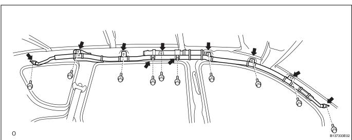
(a) Install the curtain shield airbag with the 10 bolts.
