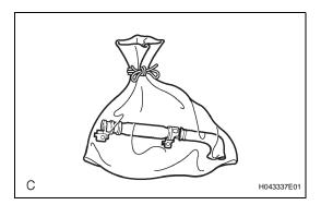
(3) Press the SST activation switch and deploy the airbag.
