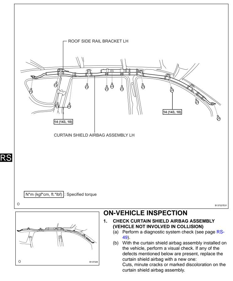
If any of the defects mentioned above are present, replace the curtain shield airbag with a new one. **CAUTION:**
