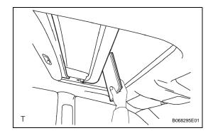
(a) When the sliding roof auto operation is operating and an object is caught between the vehicle body and glass, check that the roof glass opens a distance of 218 mm (8.58 in.) from the point of contact with the object, or opens fully if an opening distance of 218 mm (8.58 in.) is not available.
