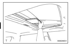
(b) When the TILT UP / DOWN function is operating, and an object is caught between the vehicle body and the roof glass, check that the sliding roof tilts up fully.
