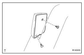
(b) Install the cover with the 2 screws.
