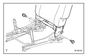
INSTALL REAR NO. 1 SEATBACK ASSEMBLY RH (w/ o Rear No. 2 Seat)
