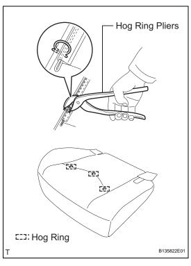
(b) Using hog ring pliers, install the seat cushion cover (with pad) to the seat cushion frame with 18 new hog rings.
