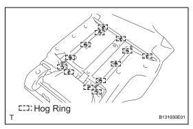
(d) Lift up the seatback cover and install the 13 hog rings.
