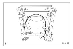
(b) Attach the 2 clamps and connect the cable to the reclining adjuster.
