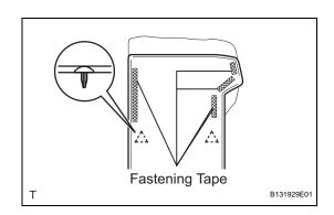
(c) Attach the 2 clips and close the fastening tape.
