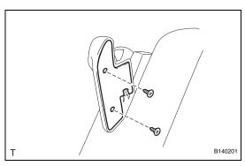
(b) Install the cover with the 2 screws.
