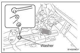
7. INSTALL REAR NO. 1 SEATBACK ASSEMBLY RH (w/ Rear No. 2 Seat)
