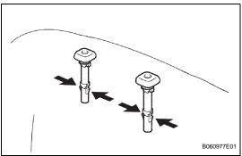
(c) Attach the 4 claws to install the 2 headrest supports.
