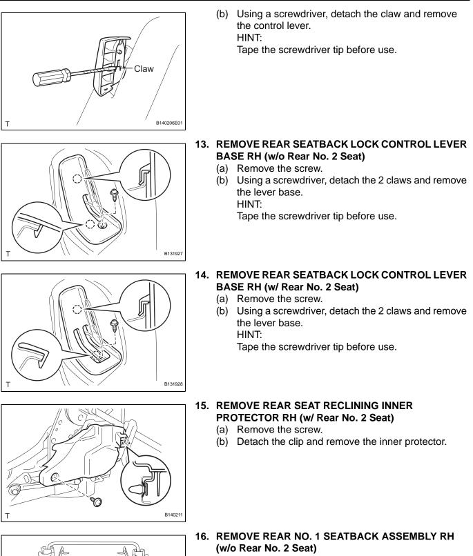
(a) Detach the 2 clamps and disconnect the cable from the reclining adjuster.
