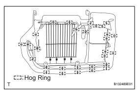
(b) Remove the 29 hog rings and seat cushion cover (with pad) from the seat cushion frame.
