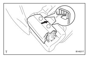
(b) Pull the armrest cover in the direction indicated by the arrow in the illustration to detach the 2 claws. Then remove the armrest cover.
