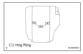
(d) Remove the 3 hog rings and seatback cover from the seatback pad.
