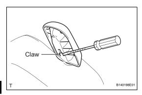
(b) Using a screwdriver, detach the claw and remove the release lever.
