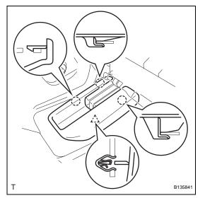
7. INSTALL REAR NO. 5 SEAT LEG SIDE COVER(a) Attach the 3 claws and clip to install the side cover.
