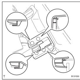
11. INSTALL REAR NO. 3 SEAT LEG SIDE COVER (w/o Rear No. 2 Seat)
