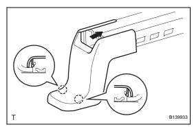
(h) Install the front seat track bracket outer cover in the direction indicated by the arrow in the illustration and attach the 2 claws.
