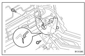
(c) Detach the 4 claws and remove the 2 headrest supports.
