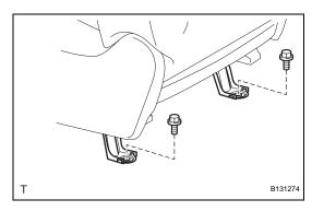
(f) Remove the 2 bolts on the rear side of the seat.
