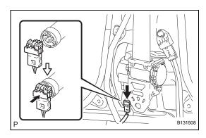
(b) Connect the pretensioner connector as shown in the illustration.
