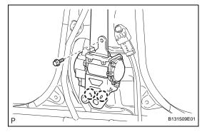
(a) Align the 2 claws with the seat belt positioning holes, and install the retractor of the outer belt with the bolt as shown in the illustration.
