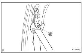
(c) Connect the outer belt with the shoulder anchor's bolt.
