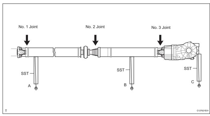
(e) If the result is not as specified, replace the center support bearing adjusting washer with a more appropriate one.
