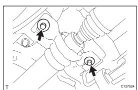
(e) Temporarily install the center support bearing and center support bearing washer with the 2 bolts.
