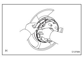
(b) Install the shoe with the shoe hold-down spring and pin.
