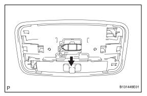
(c) Using a screwdriver, detach the 4 claws and remove the light.
