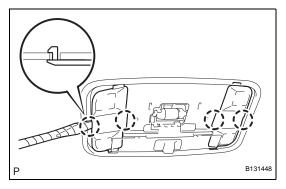
(b) Remove the bulb from the room light switch base.
